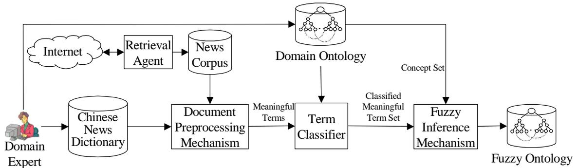
Fig. 1. The process of the fuzzy ontology construction [1].
